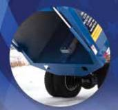
Floor is manufactured with long-wearing Hardox® 450 Steel.
