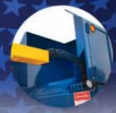
Extended debris shroud keeps refuse in the hopper.
