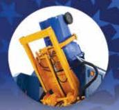
Fast cycle times, continuous packing and 50 degree minimum dump angle.
